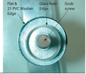
Slide Washer PVC 21 mm, then Flat washer followed by the washer PVC 12.5 mm, onto each grub screw.
