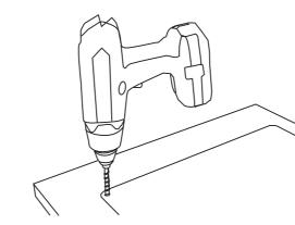
5. Construct a wood frame or use mounting clips to support the sink.
