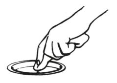
(c) Replace and rotate waste lid until it snaps into place.
