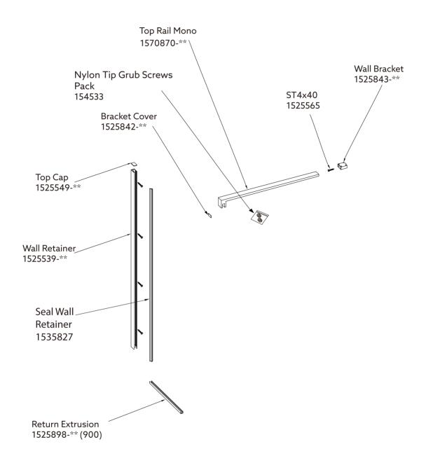
1525550 Fitting kit Wall Retainer (Bag of 9 screws) ST4 x 30 1525565 Fitting kit Wall Bracket (Bag of 2 screws) ST4 x 40
