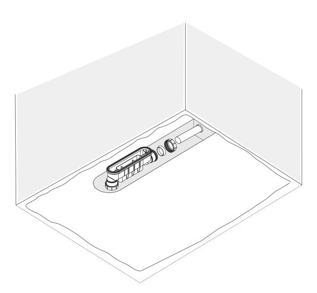
For water to drain away properly, the waste pipe must have a minimum of 18 mm per meter fall.
