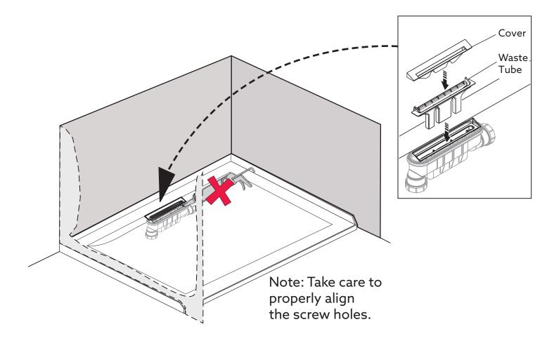
**d.** Check the waste for leaks by pouring basket of water.
