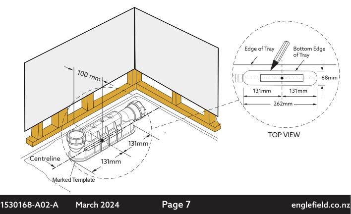
**5.** Now you have the correct waste position, measure/cut your waste pipe accordingly and fit it to the waste as detailed in the next steps (some minor adjustments may be required as necessary).
