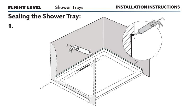
Apply silicone sealant in accordance with the manufacturer's instructions to seal the shower tray to the wall.
