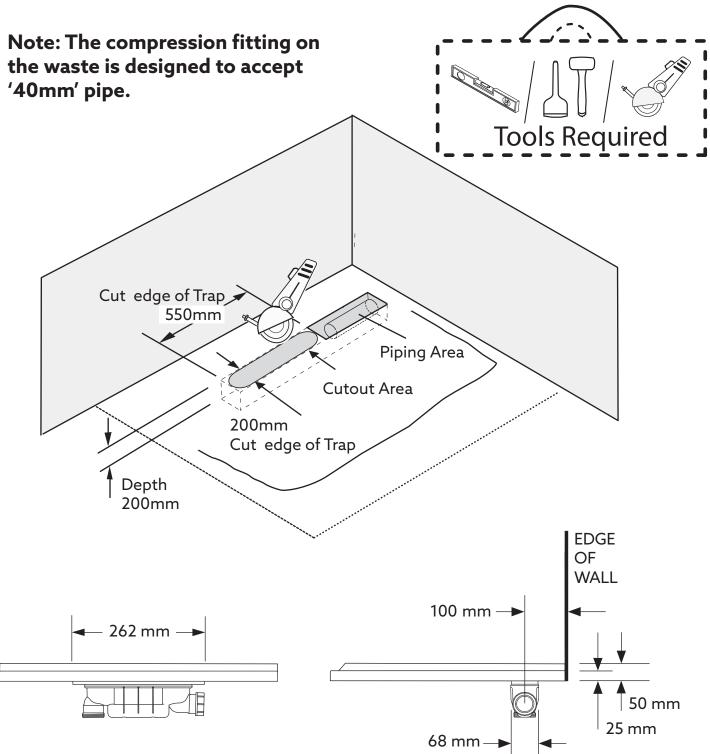
Note: If required, create an opening in the floor in order to accommodate the waste body and pipe. Make the opening oversized in order give you greater flexibility during fitting of the waste.
