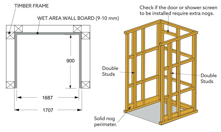
Check the fit of the tray before completing the timber frame construction. Dimensions given are nominal. Ensure there is good access to the waste fitting for maintenance.
