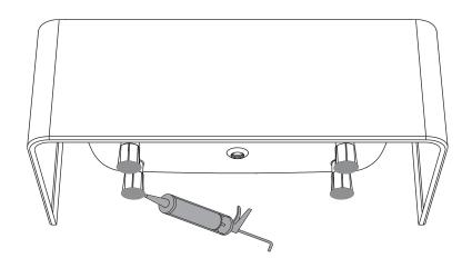
9) Apply silicone sealant between edges and adjacent surfaces ensuring that a watertight seal is formed.
