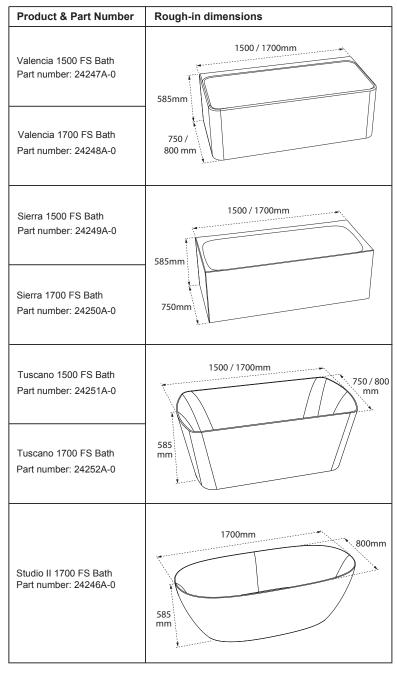
**NOTE:** Check the rough-in and room dimensions to provide adequate available space for the bath unit. Check the flooring under designated bath position and make repairs as needed. For best results, ensure that the floor is level.
