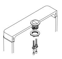
**4** Fit the lid and test the buttons. Adjust the rods as required.
