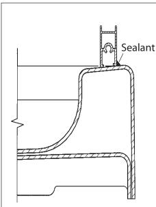
**C.** Using a fine bead of sealant, seal joint between Wall Retainer Profile and Door Assembly to a height of approx. 100 mm.
