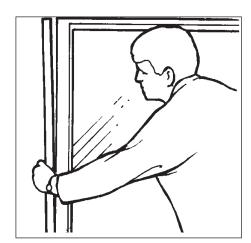
4. Slide Wall Retainer Profile into position and fix to Wall.
