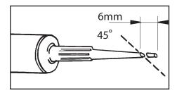
**b.** Hold the tube at 45° angle and push forward as sealant fills the joint.
