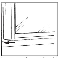
Locate the profile 10mm from the front of the shower base. Check vertical with spirit level and fix retainer to the wall using the remaining long scews. Ensure the screws go into the stud. Fit all 6 screw caps.
