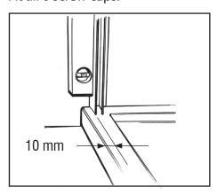
Centralise Door Assembly between Wall Retainer
