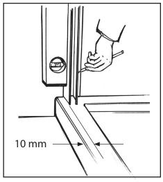
CAUTION: BEFORE DRILLING HOLES, ENSURE THERE ARE NO ELECTRICAL CABLES OR WATER PIPES BEHIND WALLS. CAUTION: We recommend fixing the wall retainers by screwing through the backing board and into studs. Other methods may cause warping and may void warranty.
