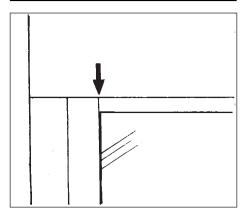
7. Using a sharp knife, trim top seal off door as shown.
