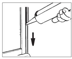
**D.** Seal joint between the Door Sill, the Return Panel and the Shower tray.
