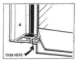
Prise drip edge seal off glass beside door edge extrusion enough to slip drip seal moulding underneath. (Note: drip seal moulding and retainer bracket are 'handed'.)
