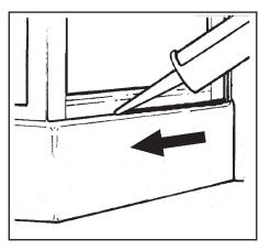
C. To a height of 100mm, seal joints between Door Frame & Corner Post and Door Frame & 180° Post.
