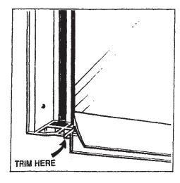
17 Prise drip edge seal off glass beside door edge extrusion enough to slip drip seal moulding underneath. (Note: drip seal moulding and retainer bracket are 'handed'.) Push drip seal firmly back onto glass and pull into contact with door edge extrusion. Clamp in place using the bracket and powder coated No. 6 screw.
