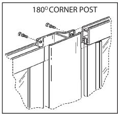
Position Infill Panel PVC gasket by pushing outside leg into both Wall Retainer & Corner Post. It should 'snap' into place.
