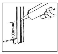
Seal up to the PVC gasket joints between Return Panel/ Infill Panel & Corner Posts and Return/Infill Panel & Wall Retainers.
