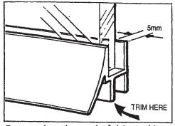
Ensure that the end of this seal just clears the Door Jamb as the door closes to create the best seal.
