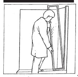
10 Fit 180° Post to Infill Panel and push into position. NB: Punched holes face inside the shower.
