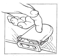
16 Slide drip edge seal over wing on bottom hinge cover and trim off at edge of glass. Repeat between hinge cover and extrusion fixed to door glass.
