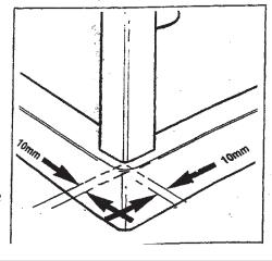
Position Wall Retainer Profiles against shower walls, resting on the shower base sill with fixing holes towards the inside of shower.
