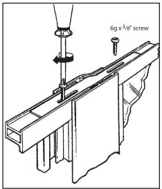
20 Using spirit level plumb Door, 180° Post and Infill Panel. Tape into position as shown. Check Door opens and shuts properly and the black lines on the Infill Panel top and bottom rails remain hidden. Readjust if necessary.
