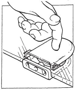
18 Slide drip edge seal over wing on bottom hinge cover and trim off at edge of glass. Repeat between hinge cover and extrusion fixed to door glass.
