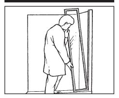
9 Fit 180° Post to Infill Panel and push into position. NB: Punched holes face inside the shower.
