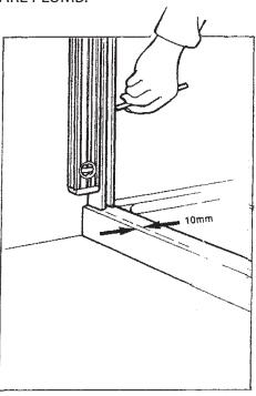
6 Repeat Step 5 for the Door Wall Retainer, <u>NOTE</u>: the fixing holes should face into the shower.
