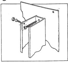
9 Insert 300mm infill panel into wall retainer so that the black mark aligns with the edge of the wall retainer. NB: The markings on the top & bottom rails should be on the outside of the enclosure & the flexible side of the PVC gasket on the inside. DO NOT push the PVC gasket into position at this stage.
