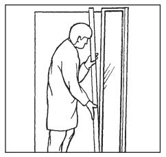
10 Insert 900mm infill panel into wall retainer so that the black mark aligns with the edge of the wall retainer. NB: The markings on the top & bottom rails should be on the outside of the enclosure & the flexible side of the PVC gasket on the inside.
