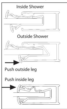
27 Fit long seal to hinge edge of glass. Flap faces into enclosure. Push down to butt against bottom seal. Trim to top of glass.
