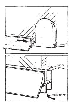
Ensure that the end of this seal just clears the Door Jamb as the door closes to create the best seal.
