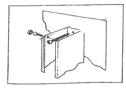
8 Insert 300mm infill panel into wall retainer so that the black mark aligns with the edge of wall retainer.
