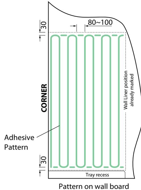
For moulded shower walls, the pattern must be marked on both wall board **and** rear of Duracryl liner. Refer to figures below for both patterns:
