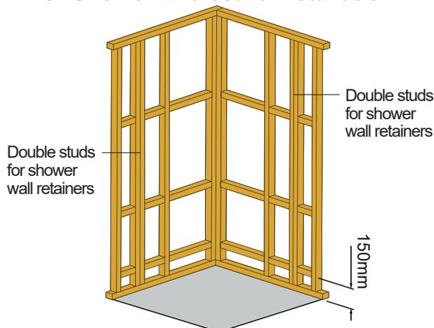
**Fig. 4: Check the fit of the wall (and shelves) prior to applying adhesive**
