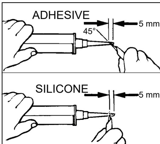
Apply sealant to shower tray or bath first as shown in **figure 15** below.
