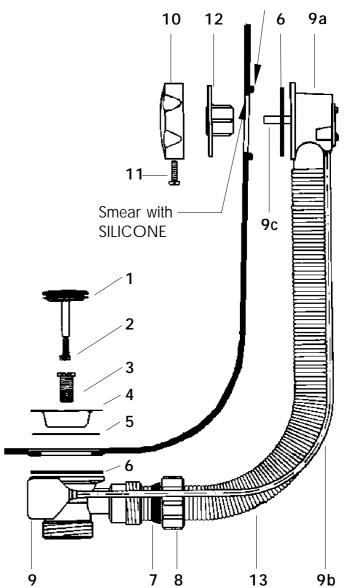
Check if the pop-up mechanism is operating correctly.
