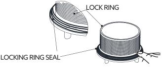
**2** Ensure the Yellow locknut on the waste outlet is tightened before completing the installation and the outlet surface is clean.
