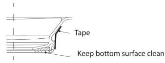
Fit the trap body with the H Ring Seal centered underneath the tray ensuring it sits flat on the Stainless Steel Cap and secure with the Lock Ring (Lock Ring Seal is pre-fitted, ref step 1). Use the Lock Ring Tool to tighten the Lock Ring against the Trap Body and achieve a watertight seal, then remove the tool, and keep for future maintenance.
