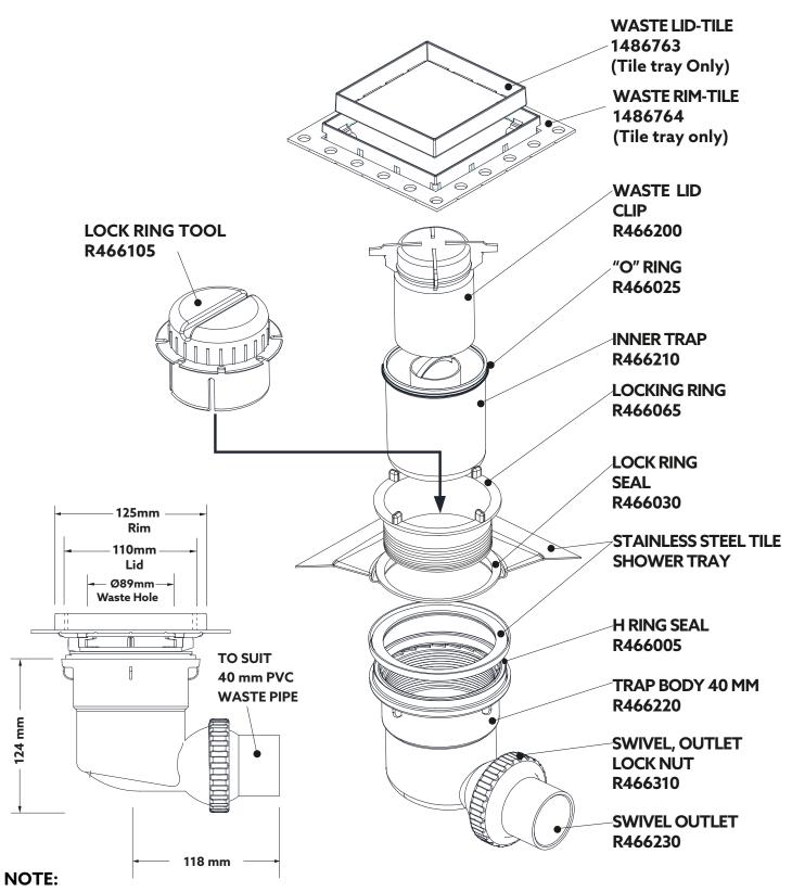
If during installation the swivel outlet is dismantled from the trap body, ensure that all parts are cleaned before reassembly.
