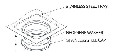
Tape lightly in position to keep the cap and washer in place during installation. Tape must not obstruct, and must allow the cap to move up freely when the waste is tightened.
