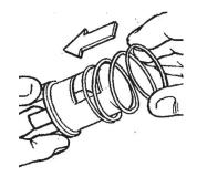
Replace the spring and sleeve into the jet body.
