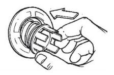
9 Re-assemble the two halves of the eyeball and fit into the sleeve. Ensure the front half is to the outside.
